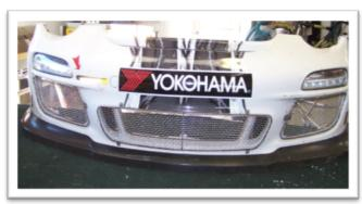
The grill screen sets for 2010 cup car nose are made of all stainless steel and the side screens cam lock. It comes with backing plates with cam lock buckets installed.
